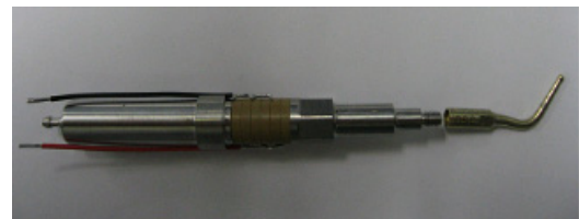
Fig. 7. Proto-sample of the ultrasonic actuator.
