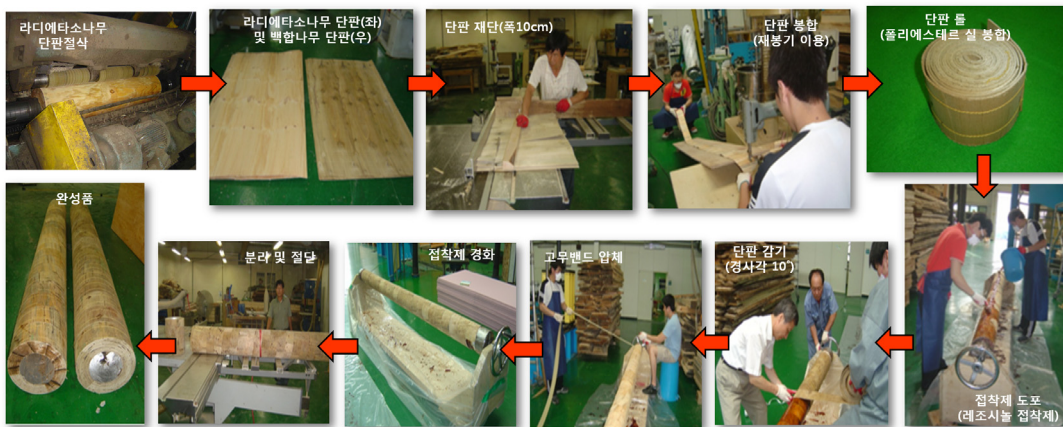
Fig. 1. Manufacturing process of cylindrical LVL.
