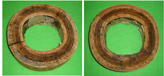
Fig. 3. The status of LVL specimen after 5 cyclic glue-line delamination test by boiling in water immersion and drying.
