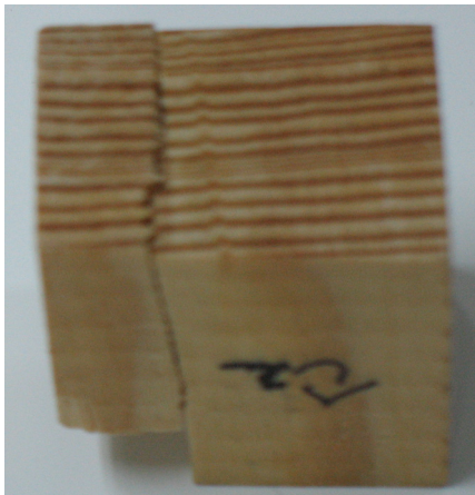
Fig. 2. Failure mode loaded by radial face for Pinus densiflora Sieb. et Zucc
