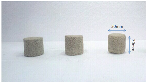
Fig. 3. Shape of specimens for durability test
