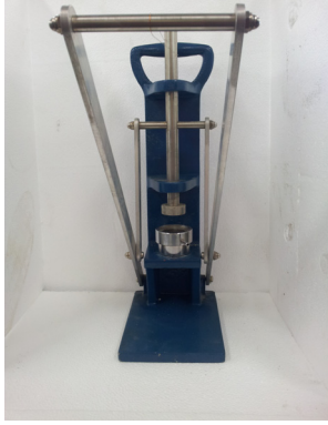
Fig. 2. Sample preparation device for durability test
