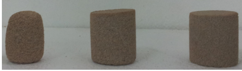
Fig. 7. Under-water cured specimens after slaking durability tests (CR = 4, 8, 12%)
