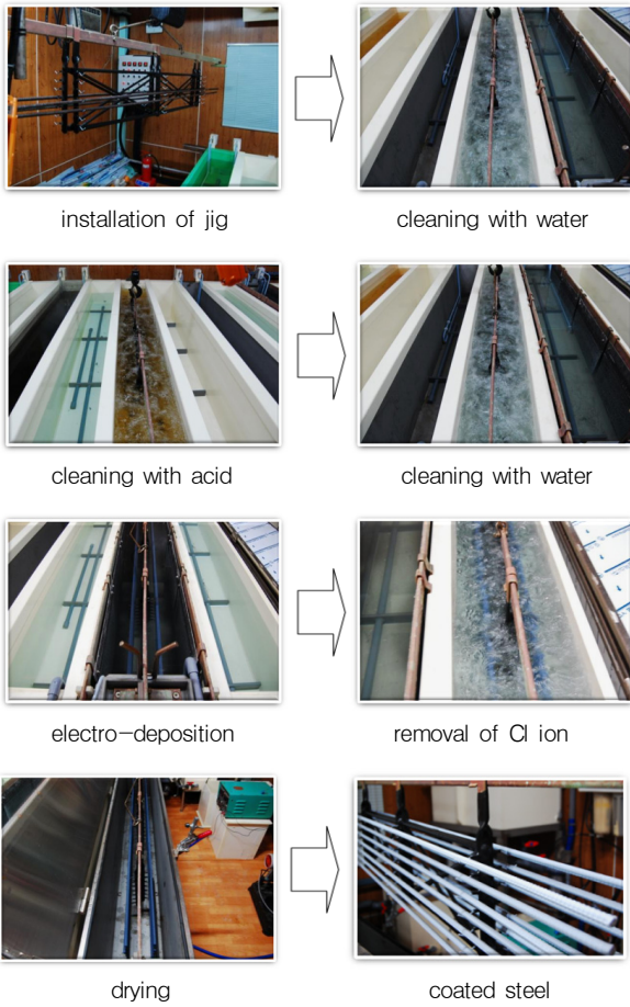
Fig. 2 Photos for steel coating process
