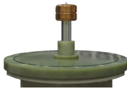
Fig. 1. Cryogenic bushing installed on big cryostat.
