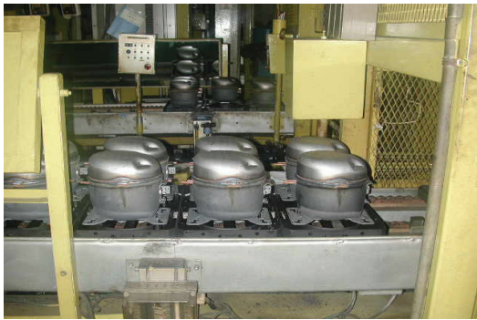
Fig. 9 Mass production line of the reciprocating compressor without health monitoring system
