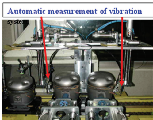
Fig. 10 Mass production line of the reciprocating compressor with health monitoring system
