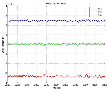
Figure 10. Measured Earth Rotational Rate w.r.t S/C Frame During the Logic Verification Test
