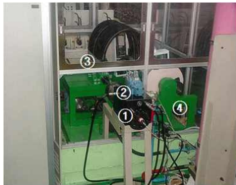
① Intensifier ② Test stand ③ Servo valve ④ Flexing equipment
