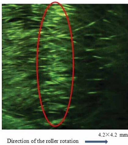
Figure 4. Snapshot of the rayon rubbing piles in contact with the substrate. Photographed with a high-speed camera.
