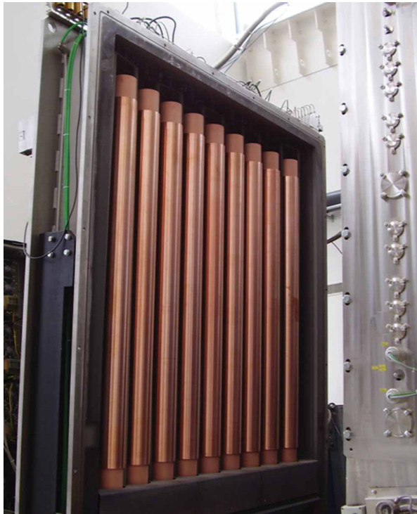
Figure 2. Typical arrangement of a rotary cathode array.
