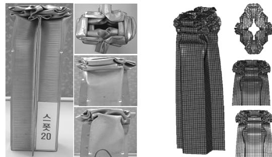
Fig. 19 Shape of experiment and FEM analysis
