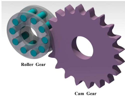
Fig. 1 RPG (Roller Pinion Gear) system
