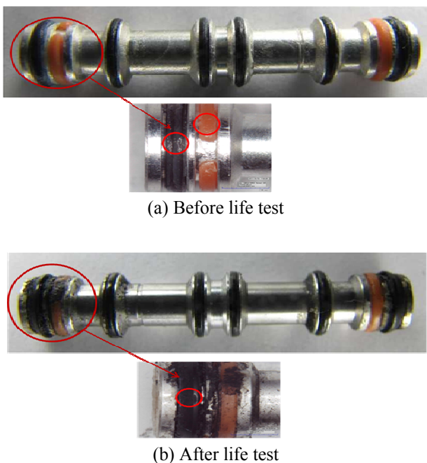
Fig. 5 Abrasion state of spool seal
