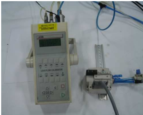
(b) Equipment of the leakage measurement test
