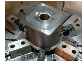
Fig. 12 A CNC machined casting and gear assembly
