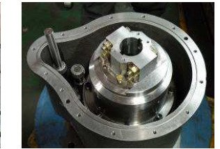
Fig. 12 A CNC machined casting and gear assembly
