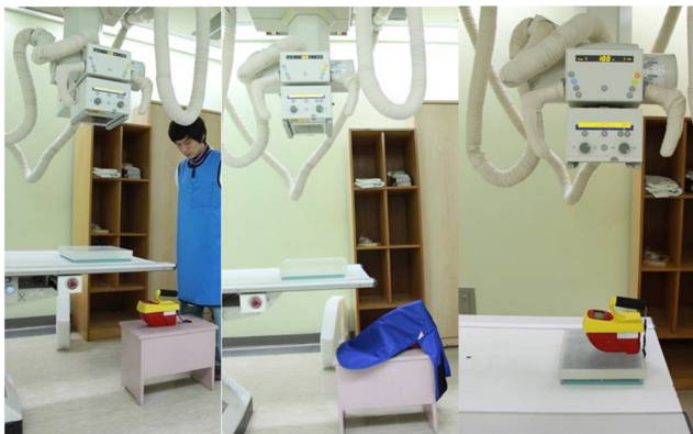
Figure 3. Measurements of radiation dose. No gonad shield(Lt.), Gonad shield(middle), Entrance surface dose(Rt.)
