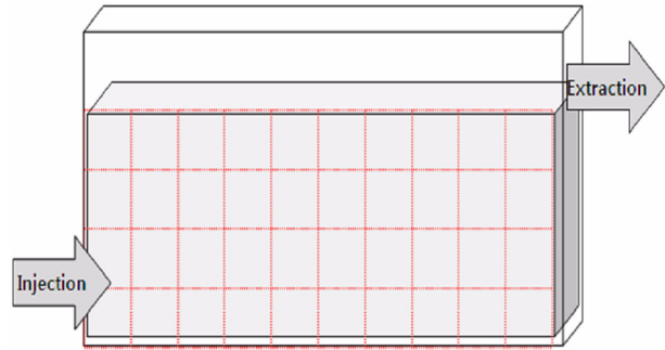
Fig. 1. Schematic diagram of experimental apparatus for 2-dimensional soil flushing (width : 70 cm, depth : 10 cm, height : 50 cm).
