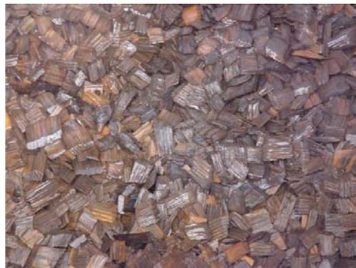
Fig. 2. Wood chip of using trickling filter system.
