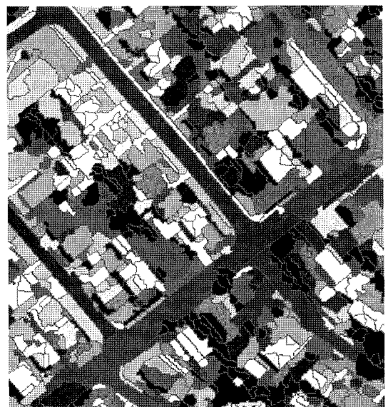
Fig. 2. The main features of road object in the segmented image.
