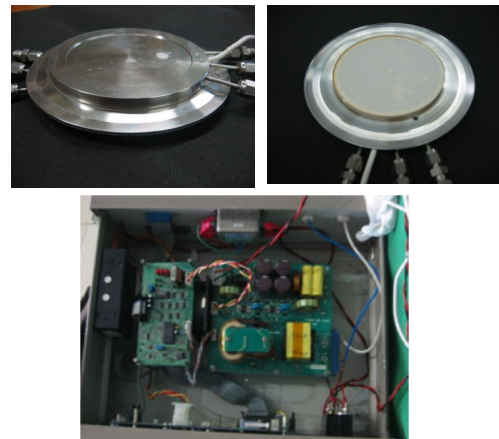
Fig. 3 Developed unit discharge cell & power supply
