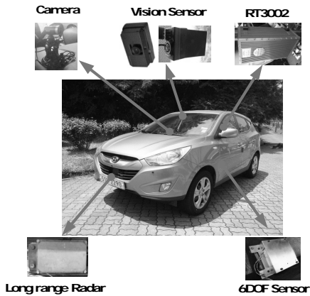
Fig. 1 Construction of experiment vehicle for road curvature data collection
