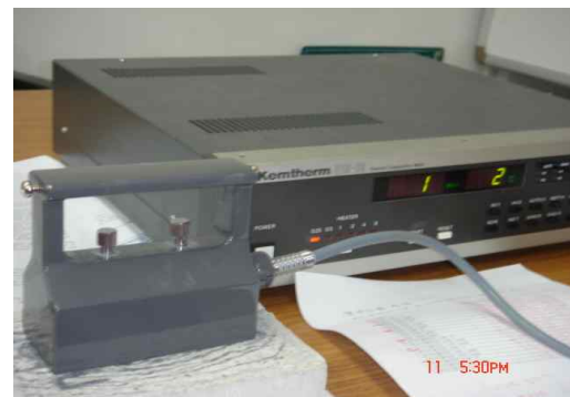
Figure 3. Thermal conductivity measurement device based on the hot wire method
