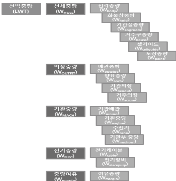
Fig. 7 Breakdown structure of the ship weight groups
