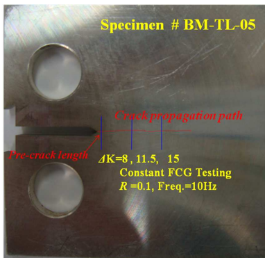
Fig. 4 Schematic diagram of FCG test for driving force
