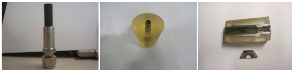
Fig. 5. Post-brazing sample preparation for SEM and EDS examination, showing brazed NiO-YSZ/316 stainless steel assembly, cold mounting of brazed assembly, and brazed assembly cut vertically and horizontally using a diamond saw, from left to right.
