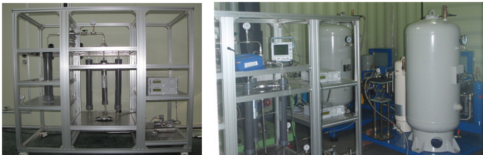
Fig. 7. Photograph of membrane pilot plant for upgrading biogas in a municipal wastewater treatment plant.
