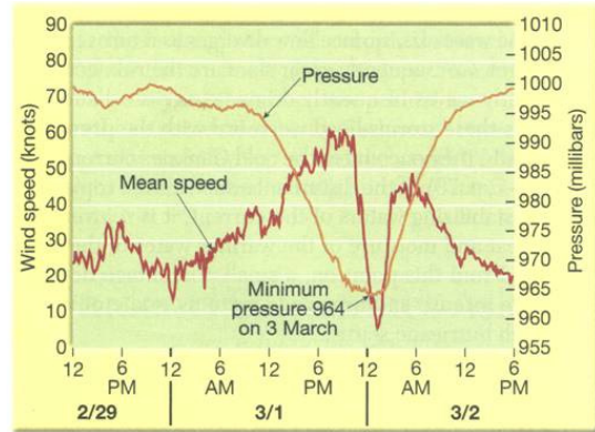
Fig. 4. Measurements of surface pressure and wind speed during the passage of Cyclone Monty at Mardie Station in Western Australia between February 29 and March 2, 2004. The strongest winds are associated with the eye wall, and the weakest winds and lowest pressure are found in the eye(Lutgens et al., 2007).
