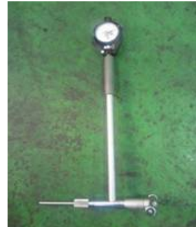
Figure 12: The diameter gauge with 1/100mm accuracy (MITUTOYO)
