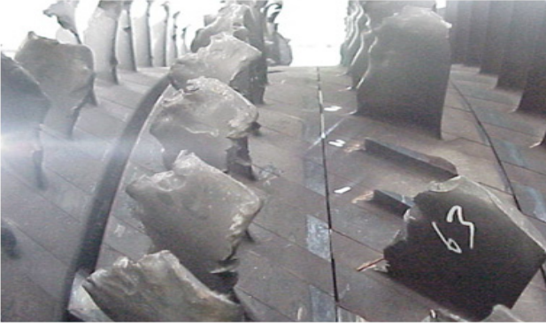
Fig. 2 Rotor blade trouble by vibration
