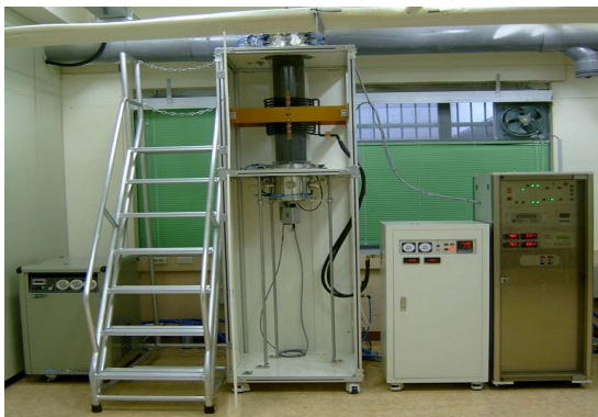
Fig. 2. A vertical furnace for the silicon carbide growth.
