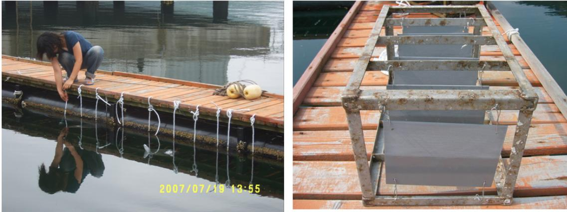
Fig. 2. The experimental platform and artificial substrates (PVC plates) in the study site (Jangmok Bay).
