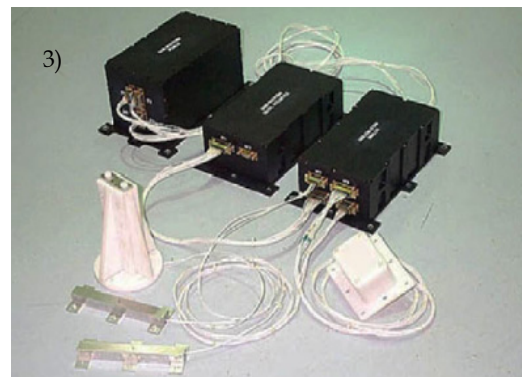
Fig. 10 The 1 UV radiometer system, 2 LP(Lang -muir probe)/ ETP(electron temperature probe) system KSR series, and 3 Magnetometer system onboard the KSR-III [7]
