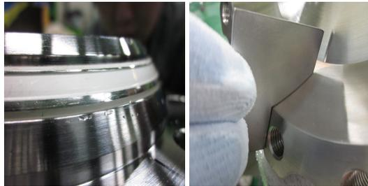
Fig. 9 Surface of the Metal Seal and Guide Plane of the Female Flange after Tests
