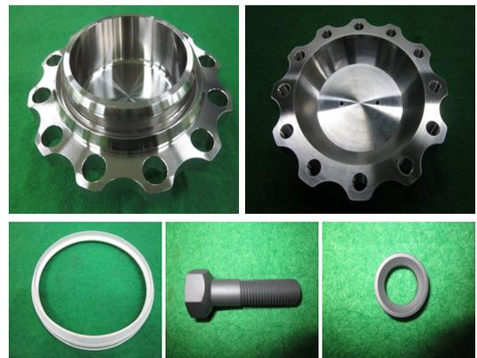
Fig. 5 Prototype of the Spherical Flange
