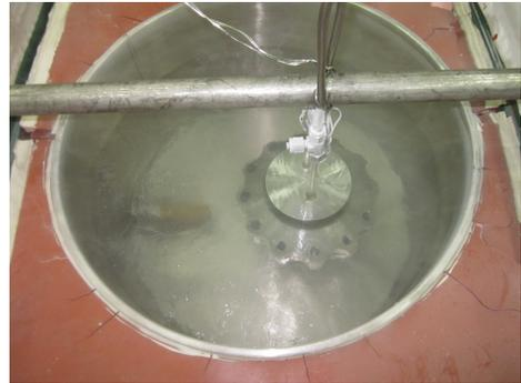
Fig. 7 Leak Test at the Cryogenic Temperature
