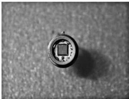
Fig. 3.4 Implementation of dual MOSFETs for a dosimeter
