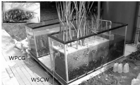
(a) Woodchip media of the vertical cartridge
