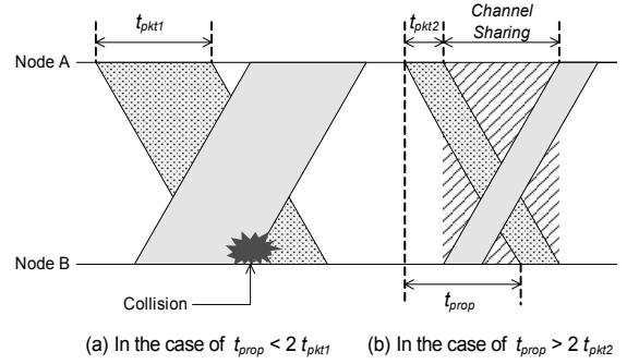
Fig. 1. Bi-directional transmission between two nodes.
