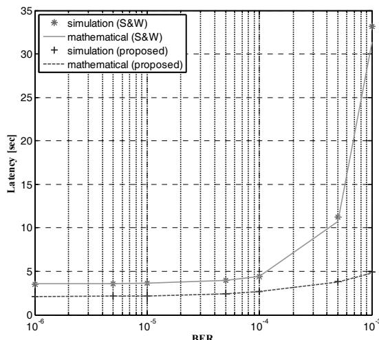
Fig. 4. The latency versus the bit-error rate.
