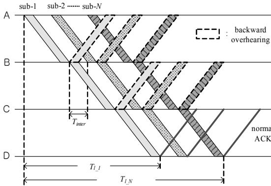
Fig. 2. Operation of the proposed ARQ scheme.
