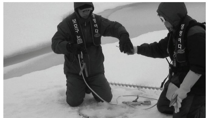
Fig. 6 Ice gauge to measure ice thickness.
