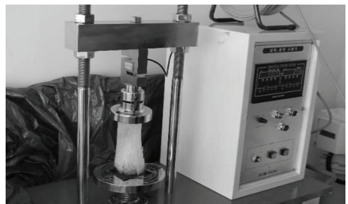
Fig. 7 Measuring compressive strength for ice specimen.
