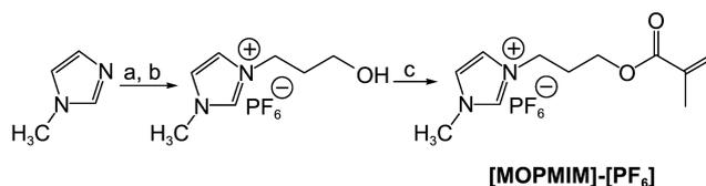
**Scheme 1.** Synthesis of [MOPMIM]-[PF<sub>6</sub>] 2d. a) 3-chloro-1-propanol, 70°C, 1d. b) hexafluoro phosphoric acid, rt., 6h. c) methacryloyl chloride, rt., 1d.
