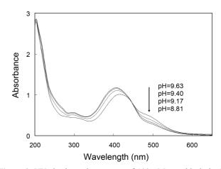
Figure 3. UV-vis absorption spectra of  $109 \ \mu$ M catechin in basic buffer solutions 19 hours after the addition of catechin to the buffer solution.
