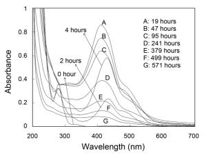
Figure 2. UV-vis absorption spectra of 91  $\mu$ M catechin in a buffer solution at pH = 8.81 at various times.
