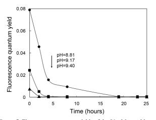
Figure 5. Fluorescence quantum yields of the 91  $\mu$ M catechin as a function of the storage time at various pH values for the basic buffer solution.
