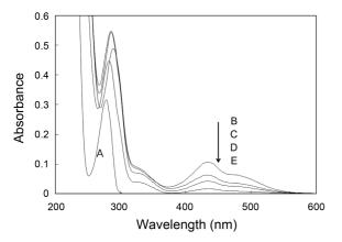
**Figure 1.** UV-vis absorption spectra of 91  $\mu$ M catechin: (a) in deaerated water, (b) in deaerated buffer solution at pH = 10.52, (c) in deaerated buffer solution at pH = 10.01, (d) in deaerated buffer solution at pH = 8.81, and (e) in aerated water.
