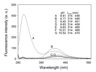
**Figure 4.** Fluorescence spectra (excitation at 280 nm) of 91  $\mu$ M catechin in basic buffer solutions 4 hours after adding the catechin to the solution.
