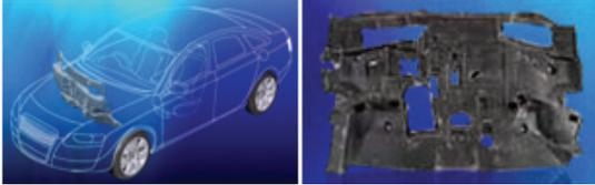
Fig. 6 Mounting position and shape of dash isolation pad
