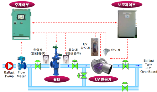
Figure 11: Configuration of the BWTS.
