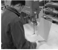
11. Processing: 3D NC processing and band-saw-in process can be used considering work efficiency and the optimized processing point of 3D NC.
