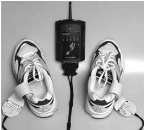
Figure 1. F-Scan Pressure Measure System 5.23
