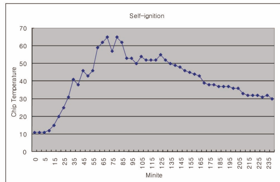
Fig. 2. Self-ignition Test after Drying Sludge-like Uranium Chips for 6.5 Hours at 300 °C under Vacuum
