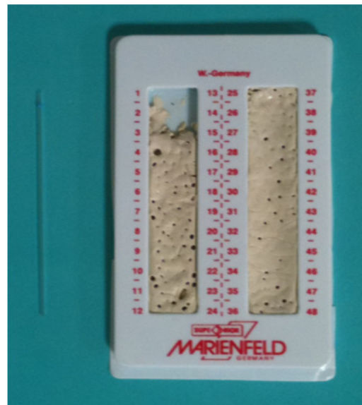
Fig. 3. capillary tube used to estimate FWHM.
