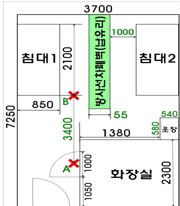
Fig. 4. Draws floor plan related to the distance between pollutions in the hospital floor and patients
