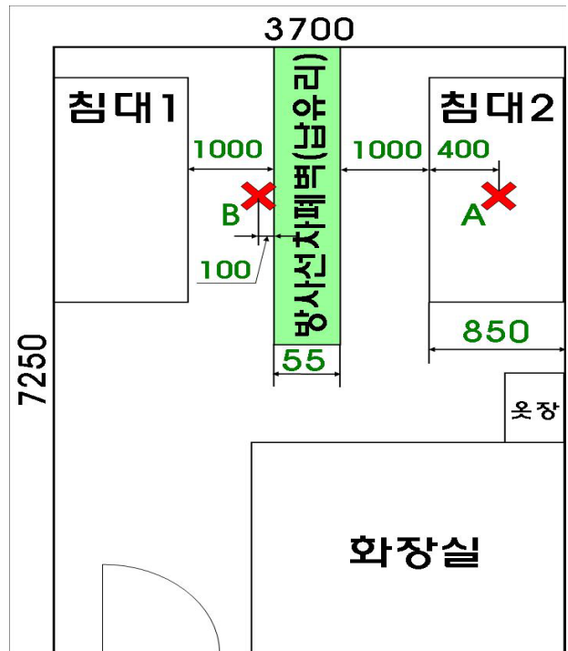
Fig. 3. Draws floor plan related to the distance from contaminated beds or patients
