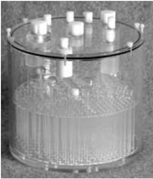
Fig. 1. The flangeless Esser PET phantom consisting of four hot cylinders was used for this study.
