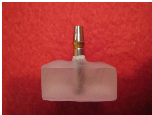
Fig. 2. Experimental specimen analog(Lab analog, GSTLA400, Osstem Implant Co., Busan, Korea) embedded in acrylic resin
