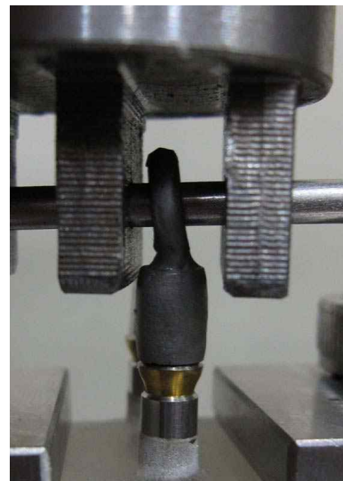
Fig. 12. Connection between testing machine and specimen
