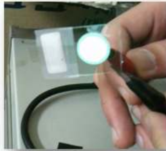
Figure 7. Electro luminescence of thin film CNT-ZnS:(Cu, Al) structure.
