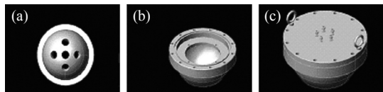
Fig. 1. 3D models of autocad drawing for multi-directional underwater CCTV camera system design. (a) rear view, (b) front view and side view, (c) completed view.
